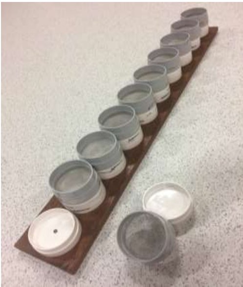
Figure 1. Scent board complete with scent pots and a detached pot with the mesh barrier PVC fitting removed (right). The location of the single target pot containing up to two myrrh-infused cotton tips was changed between each training trial. One tip was used for assessment trials.
